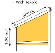
\*With a reinforced profile, the maximum fall is 2.30 m.
